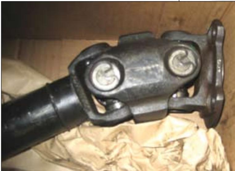
rebuild kit and 3 new U-joints (AC Delco part number 45U0168, the same as on a DI). These replacement parts do have grease fittings so hopefully I can avoid or prolong this from happening again. I did a mail order for the bearing but was able to get the U-joints at Benson's locally. You can see the old bearing in photo 3, centre top.
