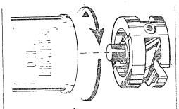
thousandth of a millimeter). Fifteen years ago, the best was about 25 microns for a full flow filter and the average was about 100. Today, an average off-the-shelf Fram filter catches particles as small as 20 microns (according to Consumer Reports, Feb. 1987 - Fram filters earned highest marks). Particles smaller than 20 microns are not considered significantly harmful by most automotive engineers.
