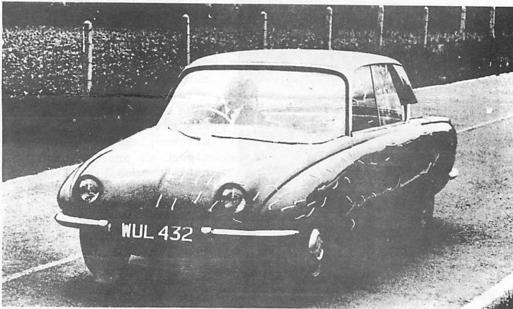
A completed prototype during one of its first outings on the Rover Company's private test track in March, 1959. The aerodynamic tapes serve to provide some indication of the air flow pattern.
