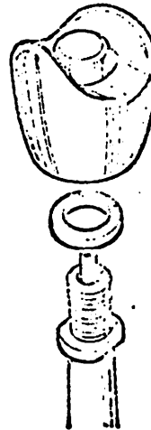
Fig. 2 Gear lever knob and fibre washer
