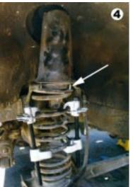
ing bolt plate will come free; if it doesn't tap it down. The freed bracket retaining bolt plate can be seen resting on top of the compressed coil spring in Photograph 4.
