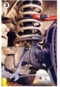
mounting bolts which are held up against the chassis mount by the coil spring. 3) The inner portion of the wing/fender sits right on top of the bracket which prevents it from being lifted up.
