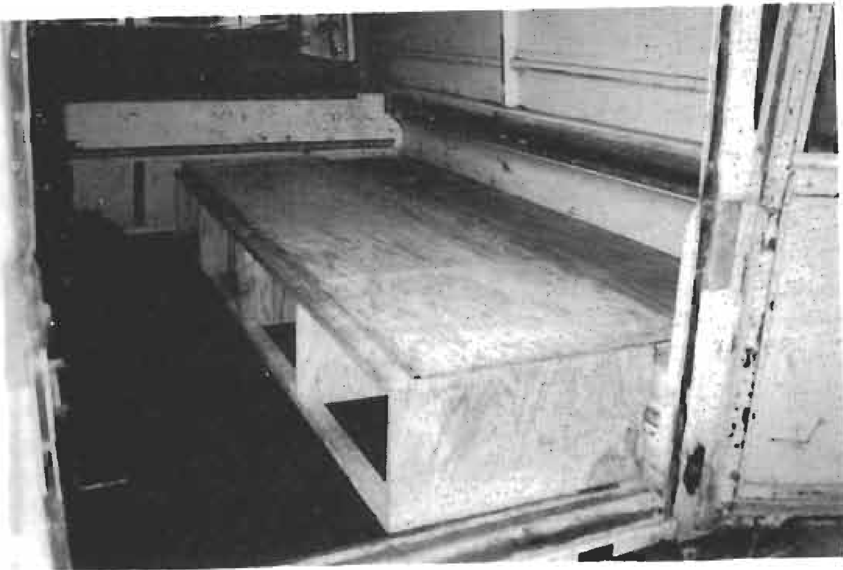
Removable bed in the 'retracted' position (platform on top) makes a good bench seat or single bed.
