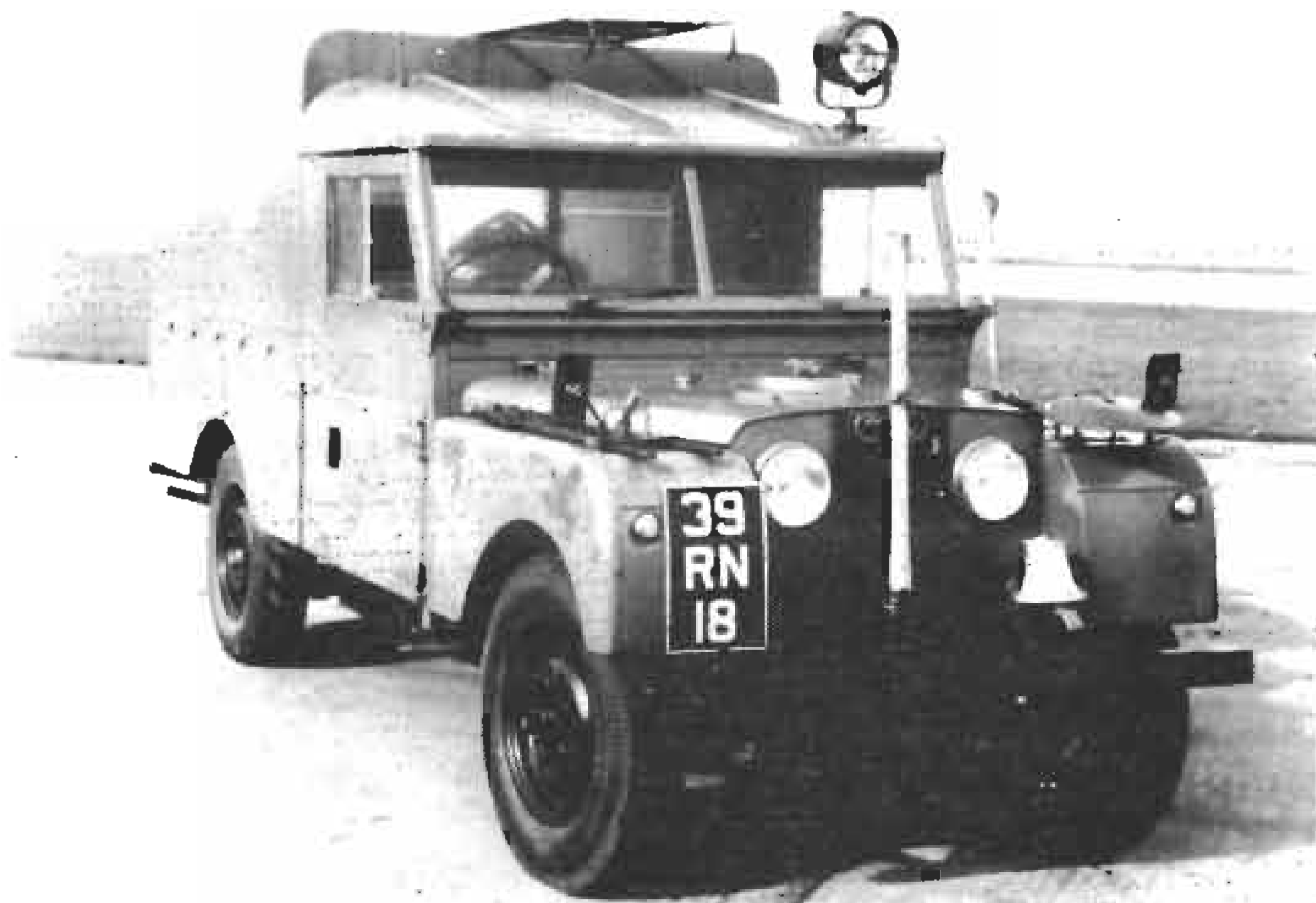
1952 Series 1 107" crash truck somewhere in the UK in service with the Royal Navy, note road tyres on the front axle, also note metal hard top for the box.
