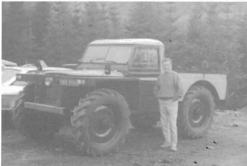
The Howat family took a trip to England toward the beginning of this year and brought back a couple of interesting Rover photos. Shown here is Jim next to a Forestry vehicle in Scotland built up a bit for things like log climbing. Those are 29" rims! And the axles have been extended for clearance too.
