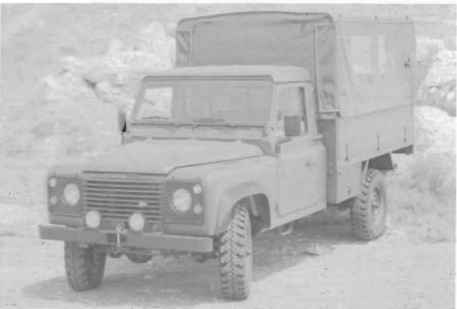
Land Rover 130", available in Turkey with several types of rear bed. This photo shows the standard 130 rear 'Hi-Cap' body. Note OTOKAR sticker on the front wing ahead of door hinge.
