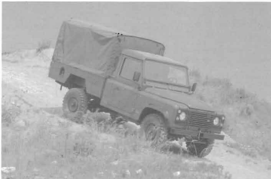
Hi-Cap, Utility, Troop Carrier, Land Rover 110" Turkish 'assembled' from CKD kit. Bench seats in rear bed accommodate 6 personnel facing inward. Photos – OTOKAR, Istanbul, Turkey.
