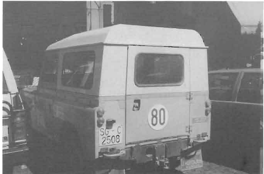
The Spanish Land Rover 'Santana' has some distinguishing marks. The reinforcement for the top in the front view and the rear door in the rear view can easily be seen here. Photo, Cliff Johnson, OR.
