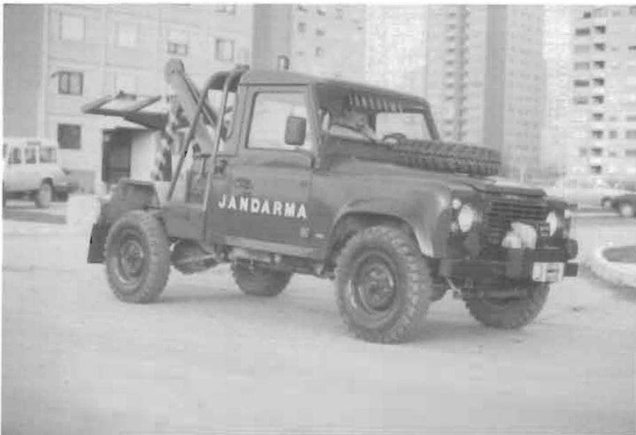
Turkish police 110" Tow Truck. Note the Warn M8274 Heavy Duty 8,000lb winch and roller fairlead on the front.
