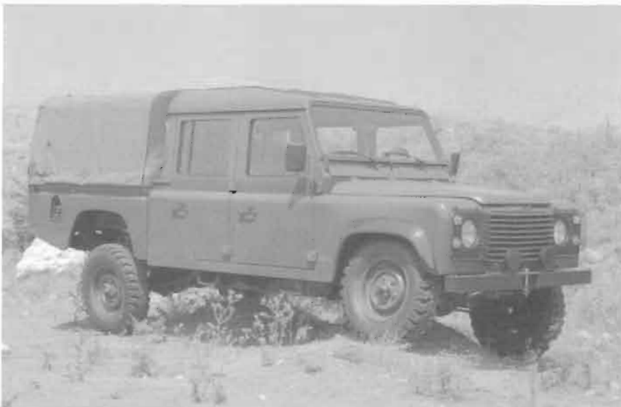
Land Rover 130" Troop Carrier available with 2.5 liter 4cyl or 3.5 liter V-8. The 130 carries a total of 12 personnel. The 10 in the rear bed sit back to back facing out.
