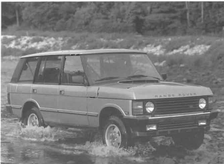
A promotional photo of the new Range Rover County LWB. The electronic Air Suspension will raise the vehicle 16 inches with the push of a button, allowing it to wade through water 22 inches deep.
