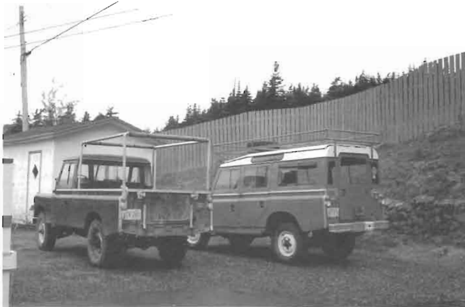
NEWFOUNDLANDROVERS is a club for Newfoundland Rover Owners. Founder, Kevin Burton owns the station wagon on the right. On the left is a series IIA 109 with a 6cyl. Chevy engine.
