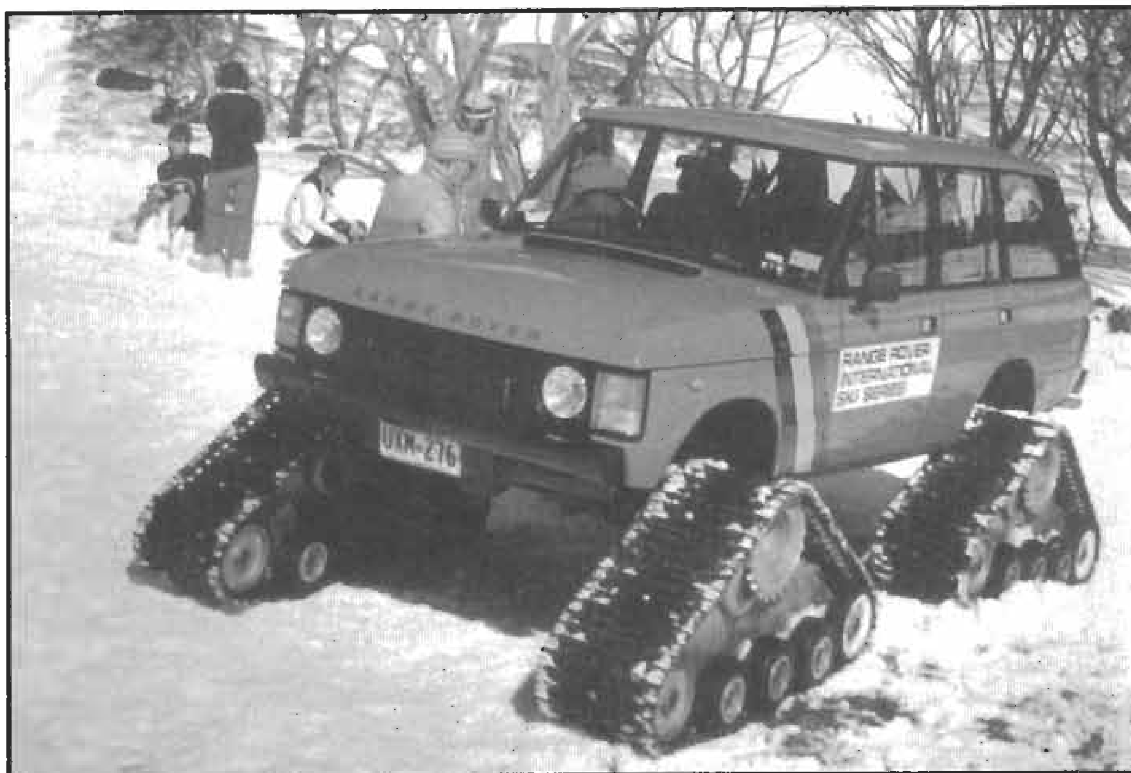
Tracked Range-Rover from Jaguar-Rover, Australla. Similar concept to early 60s Cuthbertson Conversion for 88s and 109s. Printed courtesy of LRO Magazine.
