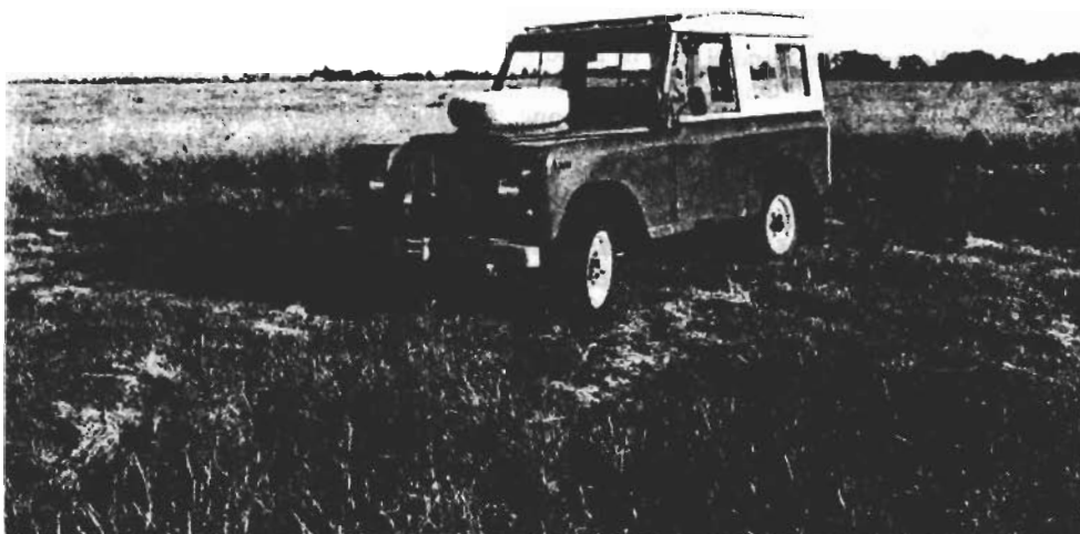
Wheelbase is 88 inches, width is 66 inches, height 77 inches and it has a 7-inch clearance.
