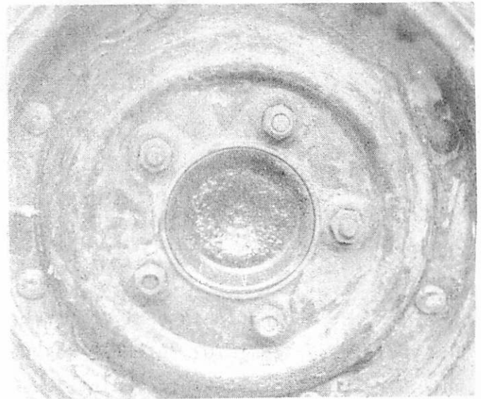
Older, semi-floating axle is at left with integral brake and hub. Newer type is in center with longer, Series II-up type in right. Above photo shows semi-float hub.
