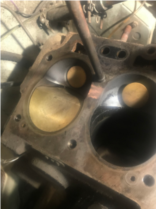
passage into #4. Plus other parts of the gasket around #4 were eroding away. The #4 piston had been steam cleaned. (Photo above and previous page. Note the difference in colour between the left piston and those to the right. Three black, one
