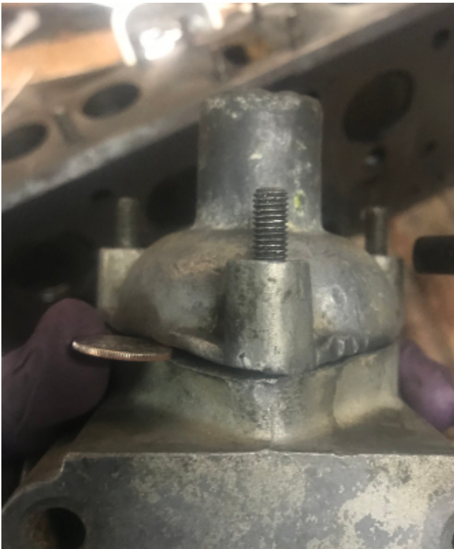
passage into #4. Plus other parts of the gasket around #4 were eroding away. The #4 piston had been steam cleaned. (Photo above and previous page. Note the difference in colour between the left piston and those to the right. Three black, one
