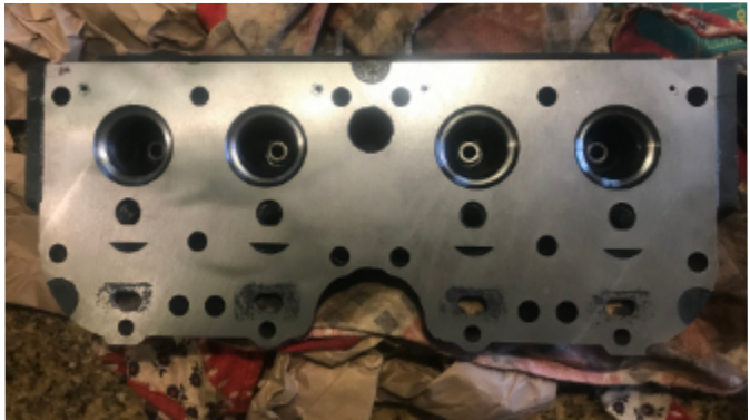
passage into #4. Plus other parts of the gasket around #4 were eroding away. The #4 piston had been steam cleaned. (Photo above and previous page. Note the difference in colour between the left piston and those to the right. Three black, one
