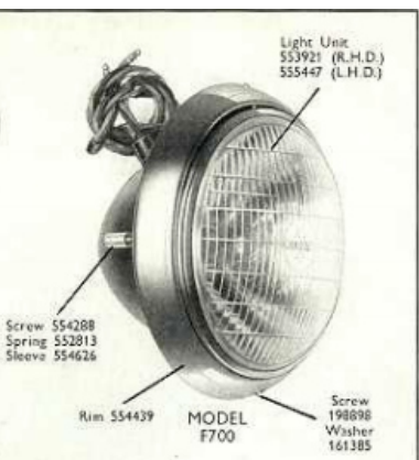
Above, the Lucas F700 unit showing the various parts. (From 1957)
