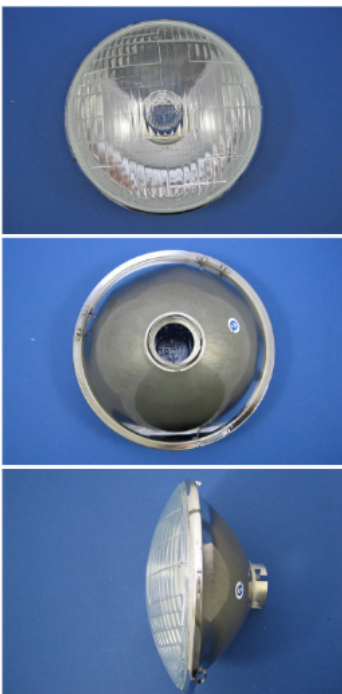
Above, the Lucas F700 unit showing the various parts. (From 1957)
