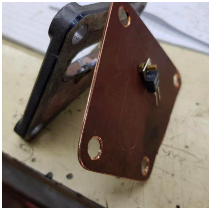
Photo 2 - replacement thermistor and copper plate
