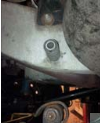
New bush ready to slide in (with a lot of help from pneumatic clamp and air gun).
