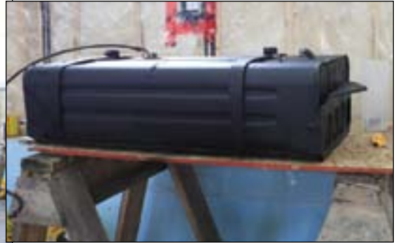
Fuel tank repaired and ready for refitting.
