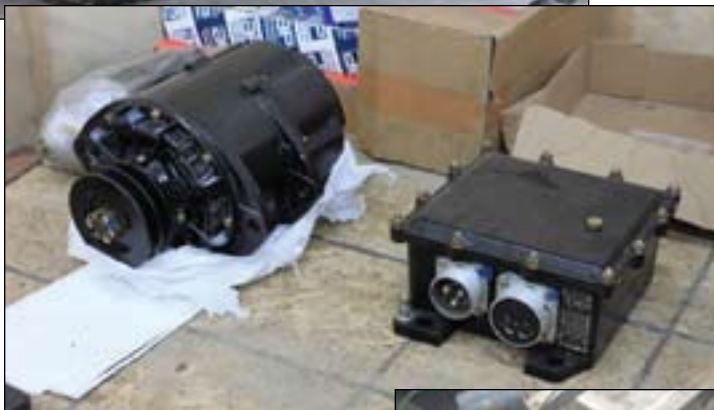
24 Volt alternator and control panel ready for refit.
