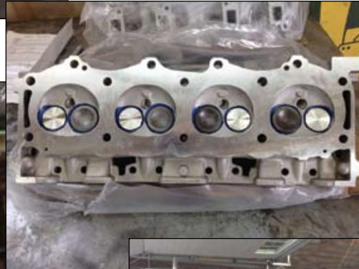
Top end rebuild in progress.
