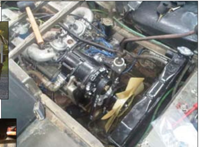
Pump alt rad belts and fan installed.
