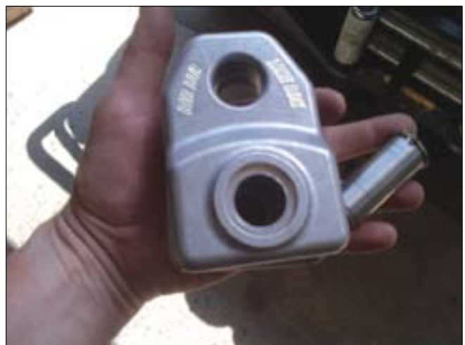
Slide out the rope retaining pin:
