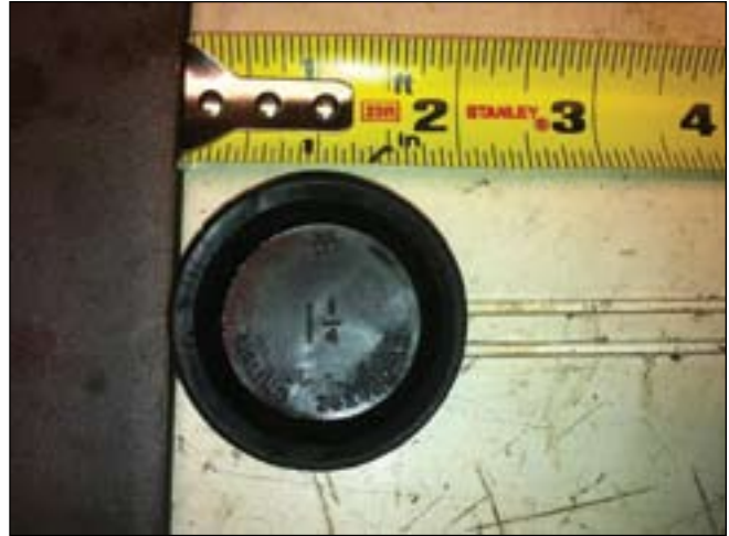
Girling Seals do expand when you use the wrong fluid. Check out the size the seal is supposed to be!
