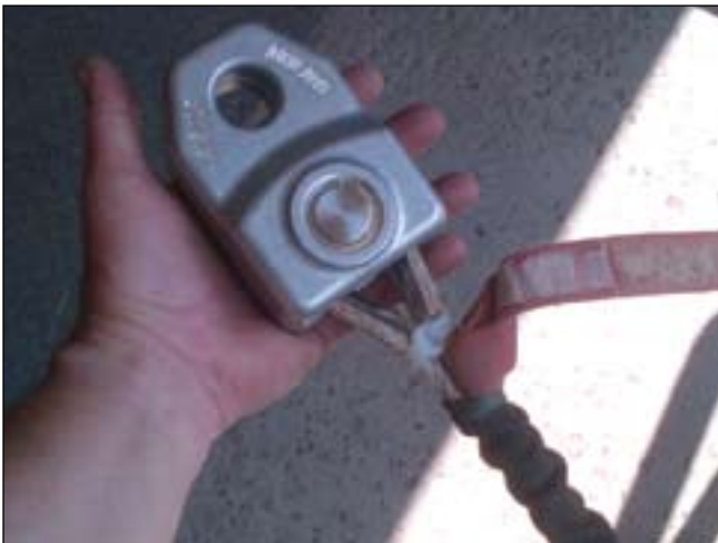
Slide the winch rope eye inside the thimble and reassemble the pin into place with the circlip:
