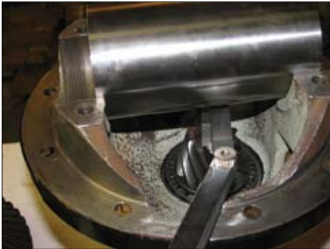
Diff Pinion height gauging with improvised gauge: 3" shaft, 2 block od 0.75" and a feeler gauge.
