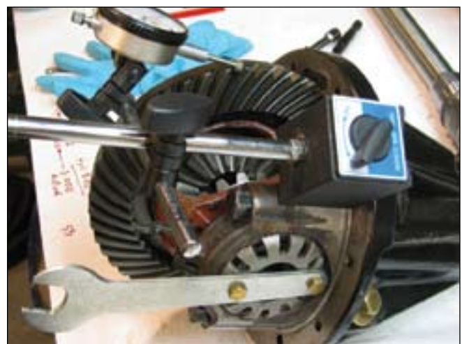
Crown-wheel back-lash adjustment with peg spanner and dial indicator
