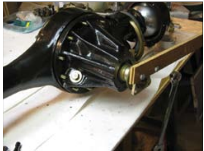
Pinion bearing preload measurement 6-10 in. lb
