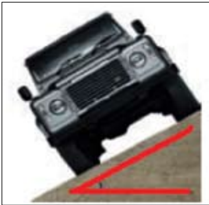
Figure 5 Maximum Traverse Angle (About 35 to 45 degrees)
