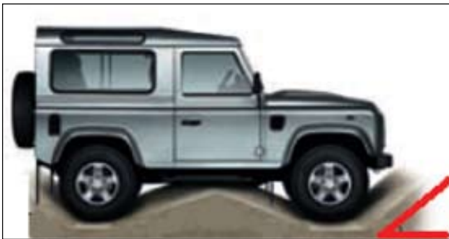
Figure 1 APPROACH Angle (Varies by model generally about 45 to 50 degrees, all figures courtesy of Land Rover)
