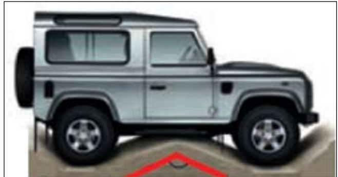
Figure 3 RAMP Angle (Varies by model and wheelbase generally about 140 to 150 degrees)
