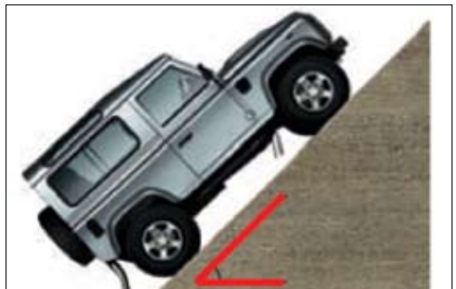
Figure 4 Maximum Gradient (About 45 to 50 degrees)
