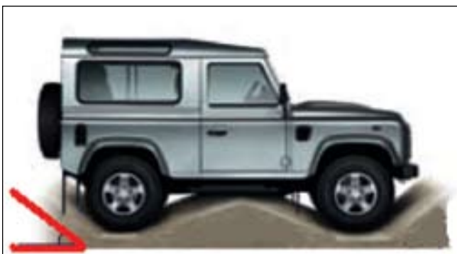
Figure 2 DEPARTURE Angle (Varies by model generally about 45 to 50 degrees)
