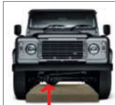
Figure 7 Obstacle clearance height (varies by model generally 10 inches at the differential)
