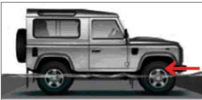
Figure 6 Maximum Wading Depth (Varies by models generally no deeper than wheel rim height about 20 inches)
