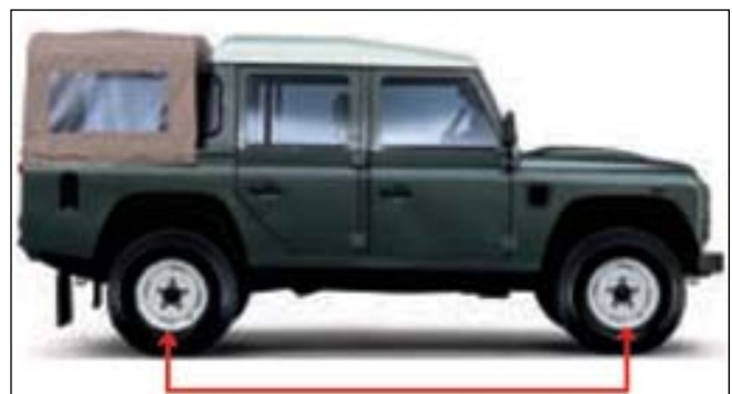
Figure 8 Wheelbase (The distance in inches between the center of the wheels, this a Defender 110)
