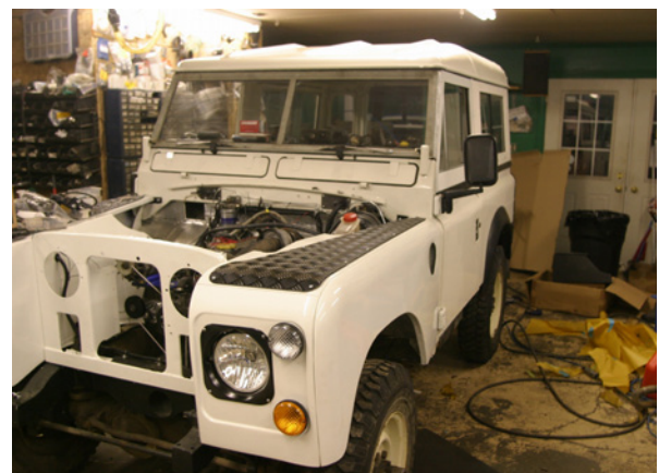
The vents are all connected; roof and door panels aligned but the bottom of the front wing needs additional braces fitted.
