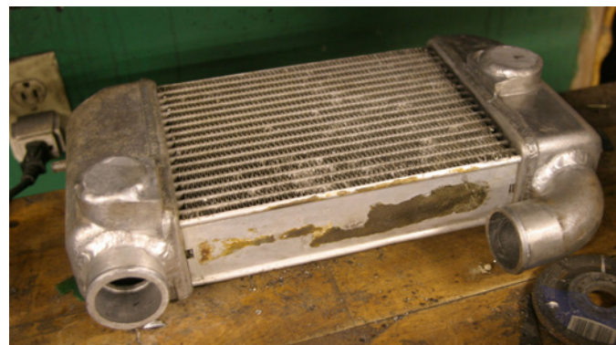
The intercooler was a particular challenge because the Series steering box sits where the intercooler would usually fit. To get things to fit a large number of custom modifications were needed including to the intercooler input/output ports.
