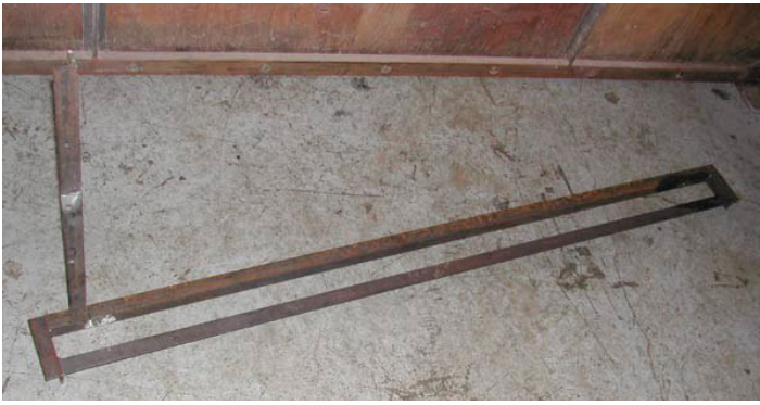
(Figure 7) Replacing the door post and ensuring an accurate fit is important. An angle iron jig should be used to ensure the correct spacing of the doorposts. A simple jig consisting of section of angle with holes in both ends which the door posts can bolt to is sufficient to ensure correct spacing.
