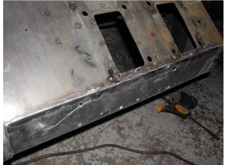
(Figure 12) The original upper panel has been attached to the replacement toe board. The weld was then ground flush so that the panels appear as though they are formed from one piece of steel as they originally would have been. When we do the other side we will detail this process a little closer.
