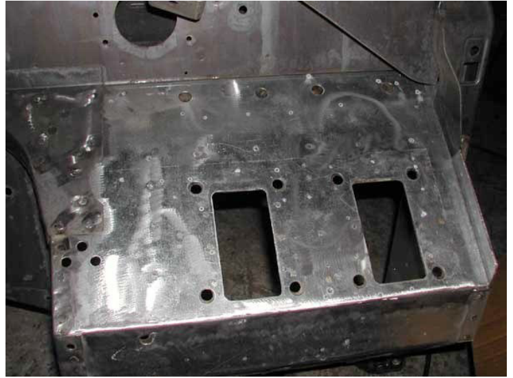
(Figure 4) On the engine side of the firewall the upper footwell is secured by the curved stiffening panel on the left hand side of the photo. The spot welds here will need to be drilled. (this photo was taken after the completed repair for reference)
