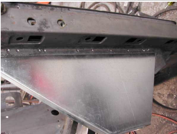
(Figure 12) The original upper panel has been attached to the replacement toe board. The weld was then ground flush so that the panels appear as though they are formed from one piece of steel as they originally would have been. When we do the other side we will detail this process a little closer.
