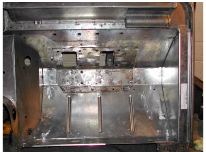
(Figure 13) On the inside of the footwell the stiffening panel has been welded into the repaired footwell. The completed assembly is constructed exactly the way the factory did it except for the now invisible seam between the upper panel and the toe board.
