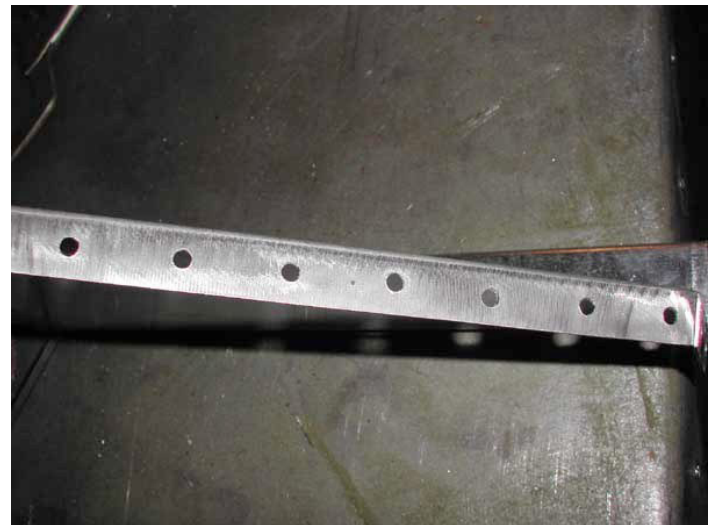
(Figure 12) The kick panel has also been drilled so that when the toe board and upper footwell are position they can be assembled with rosette welds which replicate the original spot welds.
