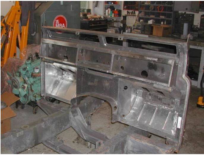
(Figure 23) Test Fitting the firewall on a frame. Thanks to the simple jig it fits perfectly and the bolts securing it to the frame slide in by hand.
