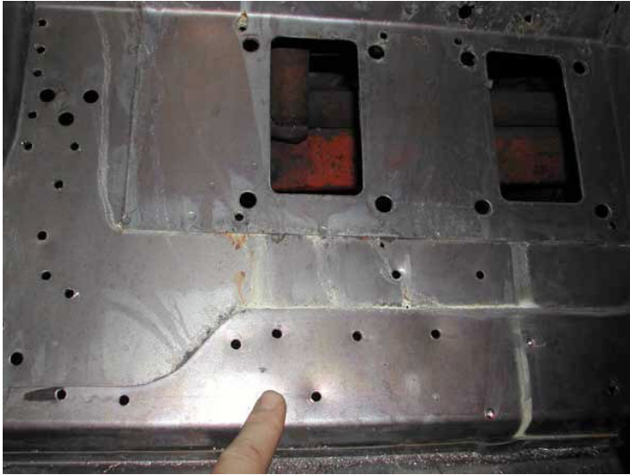
(Figure 1) The upper panel of the footwell is secured to the dash section of the bulkhead with this curved flange. If you have seen a lot of repaired firewalls you know that many times this flange is cut away along the indicated bend. This flange adds rigidity to the assembly and ideally should be retained if possible. We drilled the spot welds securing the upper footwell to this flange in order to separate the flange from the upper footwell. (The photo was taken with the bulkhead inverted)
