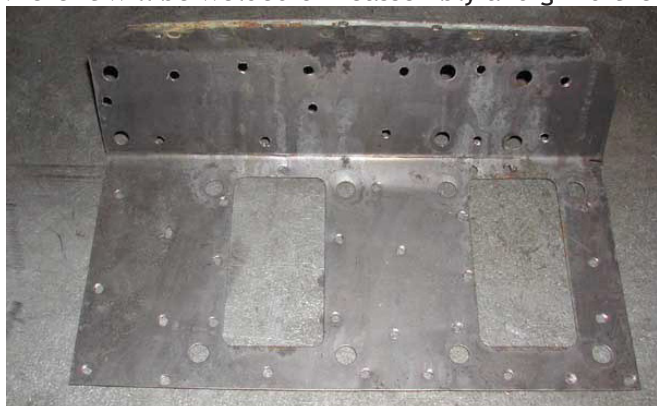
(Figure 13) On the inside of the footwell the stiffening panel has been welded into the repaired footwell. The completed assembly is constructed exactly the way the factory did it except for the now invisible seam between the upper panel and the toe board.
