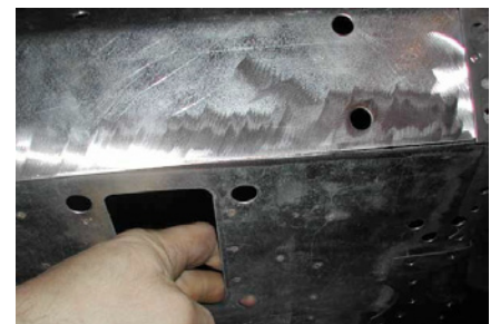
(Figure 12) The kick panel has also been drilled so that when the toe board and upper footwell are position they can be assembled with rosette welds which replicate the original spot welds.
