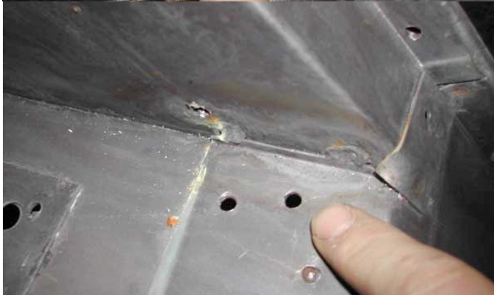
(Figures 2 & 3) On each side of this curved flange there are tack welds securing the flange to the kick panel and
