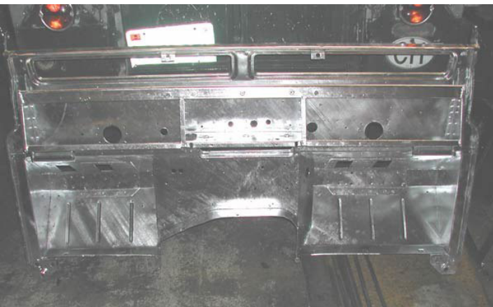
(Figures 1 & 2--above and next column) Here is the completed firewall resplendent in a fresh coat of Hot Dipped Zinc. Ready for fitment to a land rover and sure to last decades longer than a paint job!
