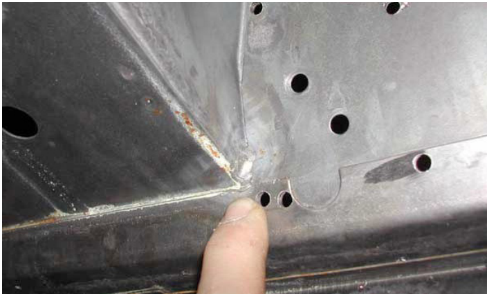
(Figure 1) The upper panel of the footwell is secured to the dash section of the bulkhead with this curved flange. If you have seen a lot of repaired firewalls you know that many times this flange is cut away along the indicated bend. This flange adds rigidity to the assembly and ideally should be retained if possible. We drilled the spot welds securing the upper footwell to this flange in order to separate the flange from the upper footwell. (The photo was taken with the bulkhead inverted)
