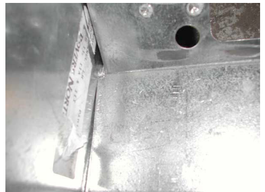
(Figure 6) A test fit of the new panels show the fit of the panels if they are not trimmed. Some minor trimming is essential to a good fit and will ease the assembly process.
