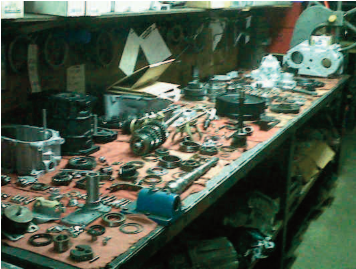
LR90 gearbox and transfer case all apart and cleaned down to the last bolt. It is stupendous how much space that it takes up compared to its assembled form.
