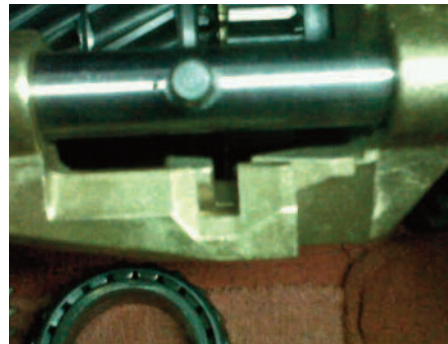
Here is the shifter fork for 3 - 4 gear as supplied, note how the notches in the centre don't line up to allow the pin to drop in and establish neutral. So now we wait for the replacement part"
