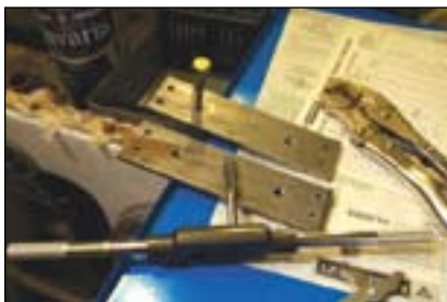
The finished products, taped for the new retaining bolts.
