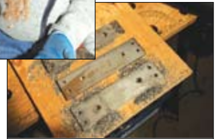
Making bracketry for the Dormatic Seats from stock steel
