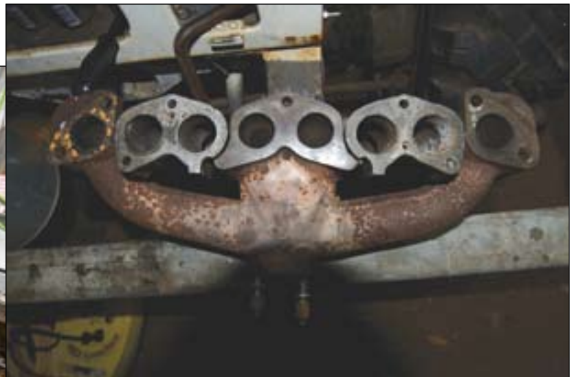
The offending manifold. Note different sized holes for the exhaust manifold..
