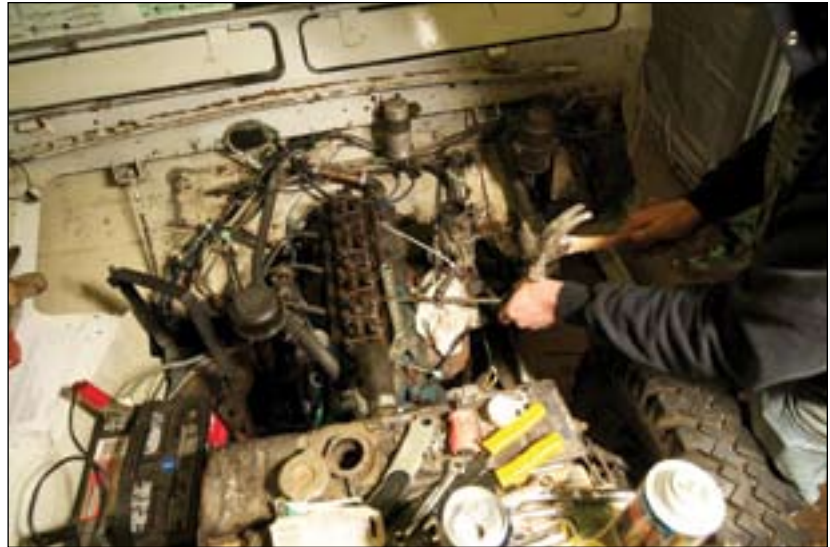
Allen trying to lever up a stuck valve on an engine that had run, but sat in the garage for about six years.
