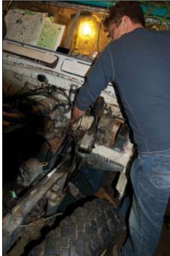
Graeme and Alastair (note, Alastair can be partially seen under Lenin) replacing the starter motor. Note tire turned to the right.
