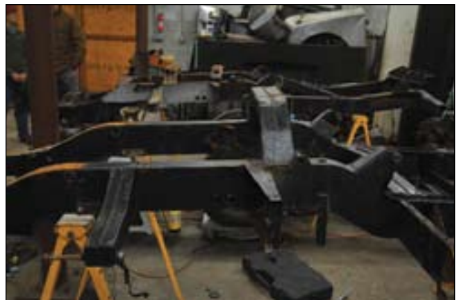
The moved engine crossmember (#2 in the #3 slot)
