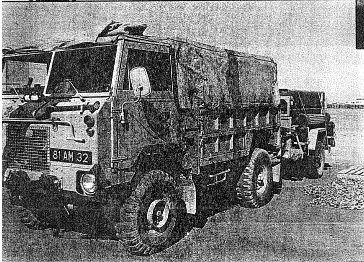
△ PHOTO C: Left hand drive One Tonne Rapier tractor belonging to 126 Squadron, RAF Regiment. Their Rovers are painted sand and green as they are operating in an area with vegetation. Note the winch pulley, front towing jaws and SA80 rifle in clip on dashboard.
