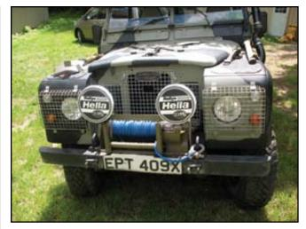
of the weight. And it came rigged with a very nice piece of kit on it. The mystery of why this winch never got used came to light when I found that a few of the pieces were missing, apparently my find had become a spares box. The 2 u-joints and pillow block that I needed to source were easily found at a local bearing shop in town. By the end of the fall 2006, I had my winch installed and ready to go but there was still a question to answer: should I use the cable or synthetic?
