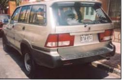
Rear view of the Daewoo Musso. Excessive overhang past rear axle hampers hill climbing but this vehicle manages fine on trails and on non-exacting off-roading.
