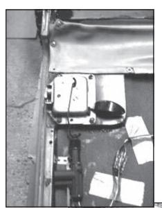
Wiring the door locks to the engine bay.
