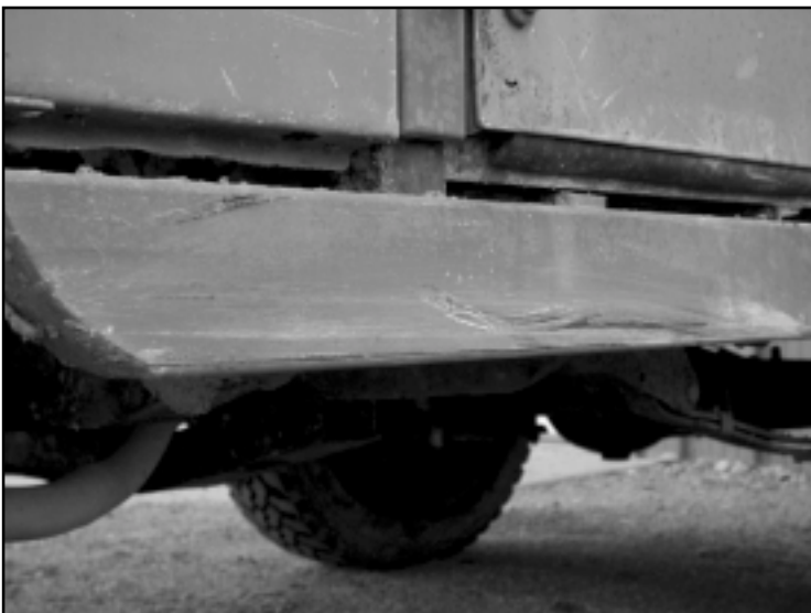
Two sliders, ready to be painted and mounted.
