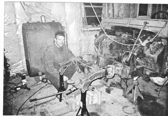
Eureka it fits! Front chassis horns from 88" tacked into place on the front of the 109".
