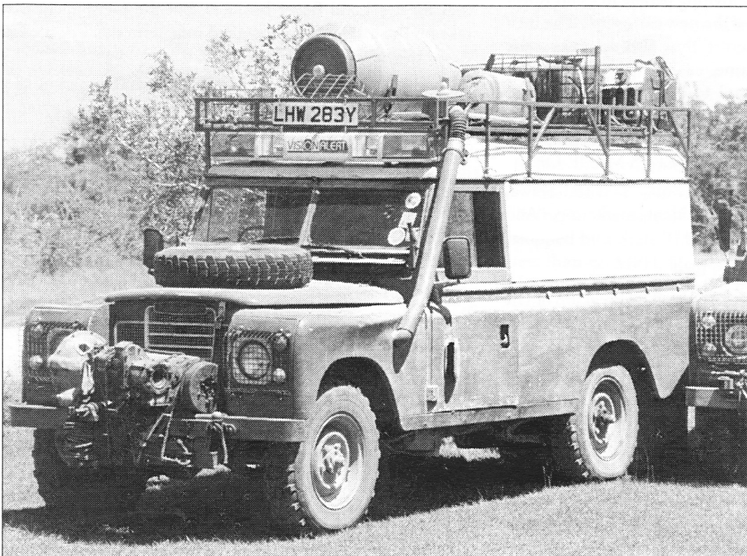
A LWB spotted on the road in Tanzania, note spare tranny mounted on bumper.
