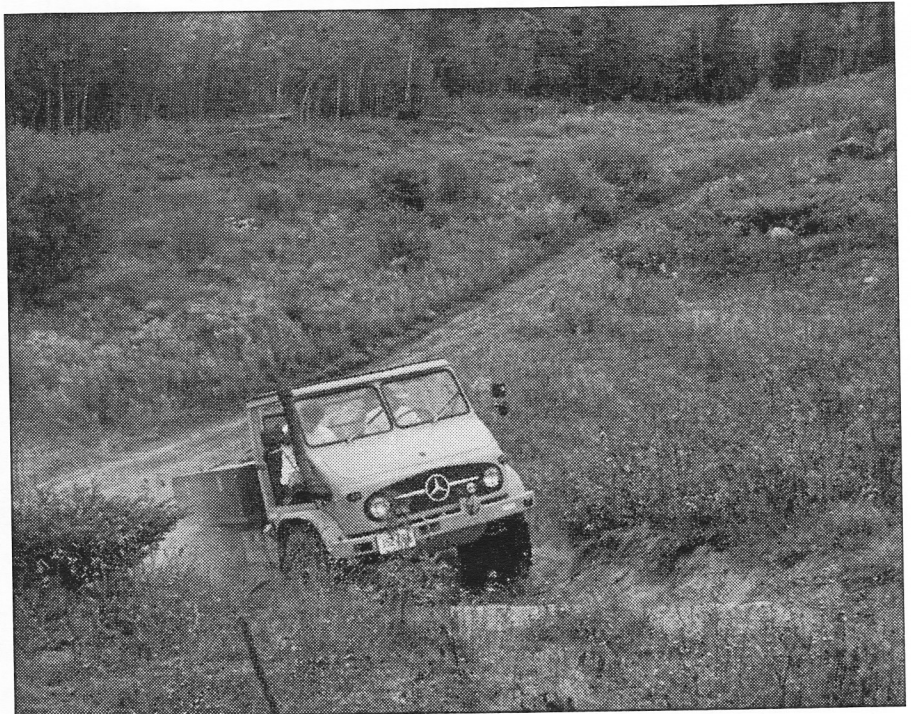
The Unimog at the hill climb, 100 feet of fine sand at a 45 degree angle.
