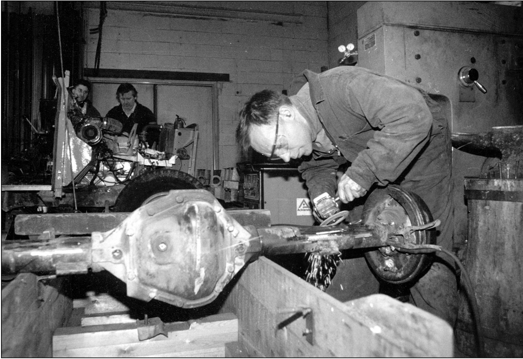
Tom ^The Torch^ Tollefson modifies the spring mounts on the Salisbury axle for fitting to the 88. Photo: Brett Storey.
