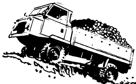
Forward Control Land-Rover with truck cab and fixed side body.
