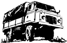
Forward Control Land-Rover with truck cab, dropside body and 3/4-length hood.
