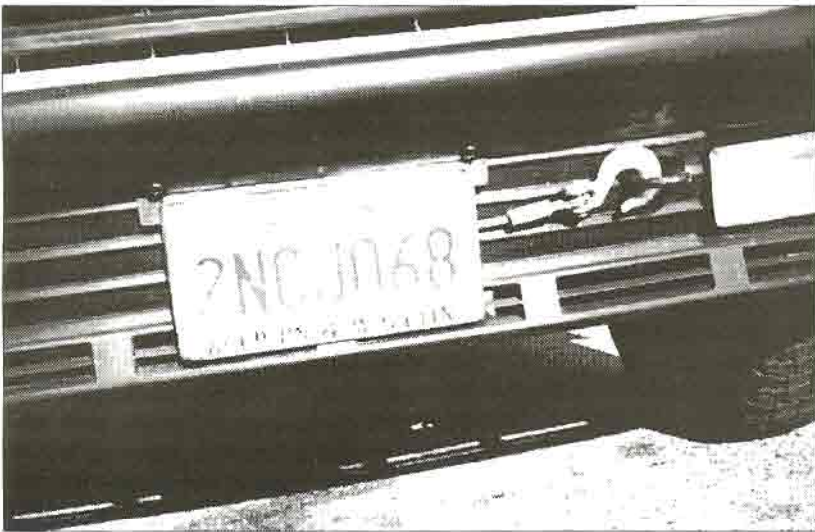
The cable end can be left out, with the hook attached to the vehicle's factory towing loop.
