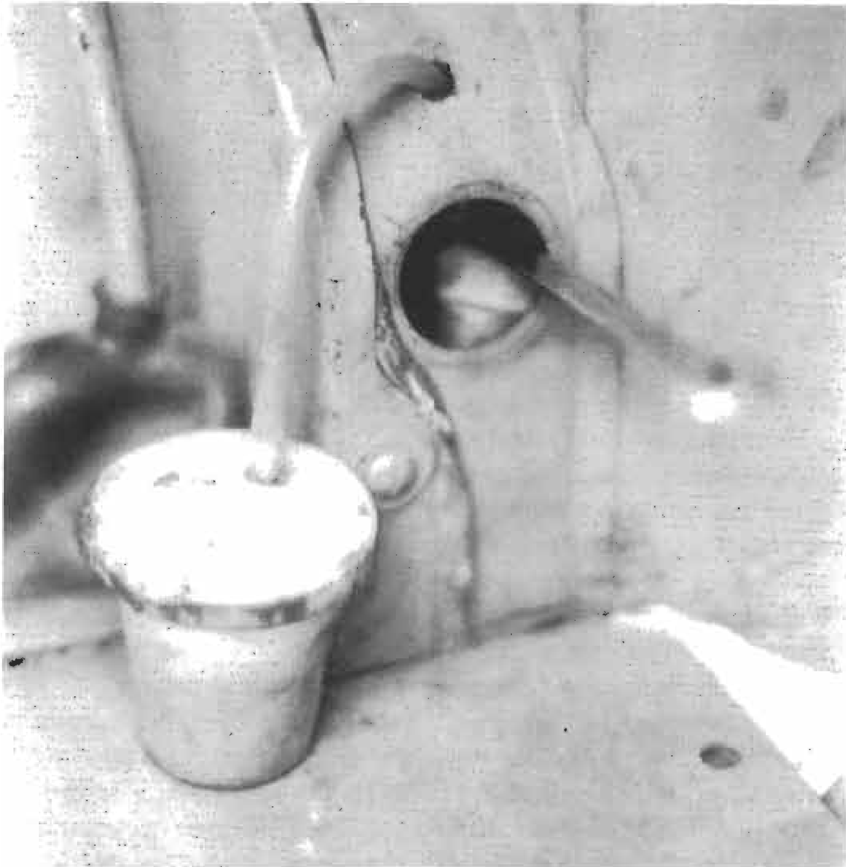
Drilling a hole into the transmission cover allows for easy clutch slave cylinder bleeding.
