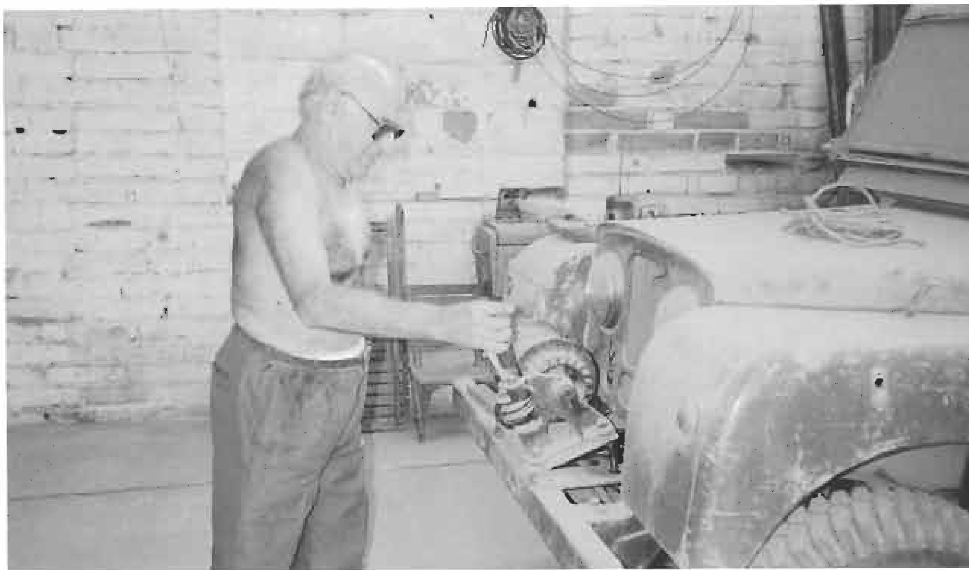
The owner demonstrates how he can rotate the whole winch out from it's 'at rest' position so that the handle won't hit the fender during operation.
