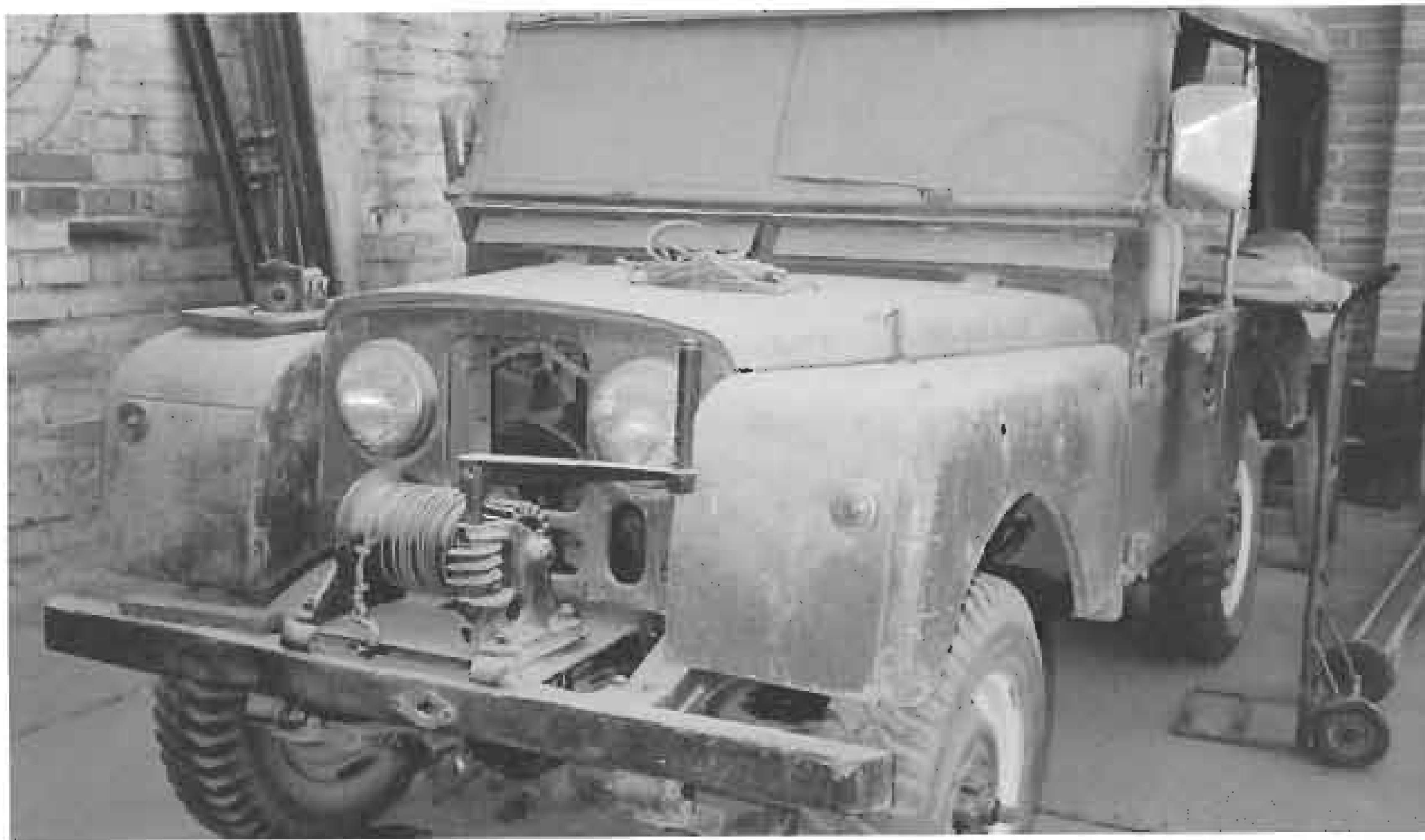
The hand operated winch is too close to the vehicle to allow the handle to make a full turn.
