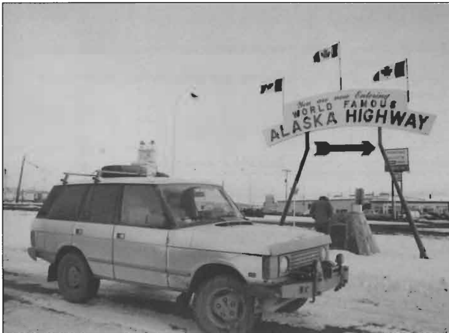
Glen's Range-Rover has a few xtras like the custom front bumper with 12,000 lb. winch attached. Probably comforting in this kind of country.
