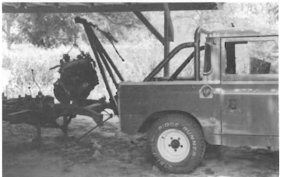
Dixieland Rovers. Ingenuity at work. A Ila with homemade hoist, a few pieces of angle iron, and a come-along lift a 2-1/4 engine.
