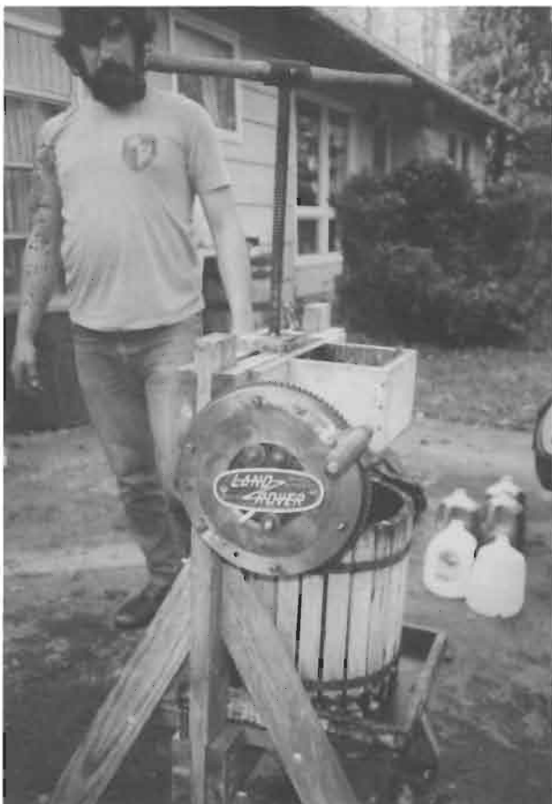
Gerry O'Brien sent in this photo of Mike Liodice (both NY). What you see in the foreground is a Rover diesel flywheel bolted onto a cider press masher for smoother hi-torque apple crushing. they say it works great!
